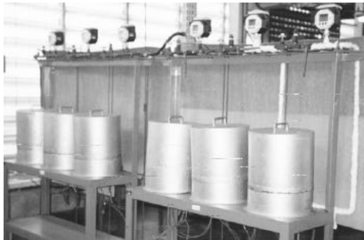
Fig.3: Class 150 and Class 300 test cells - insulated.
